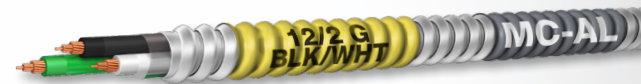
MC - THWN-2 Inners Available in 14 AWG-2 conductor through 750 KCMIL-4 conductor with or without a PVC jacket
