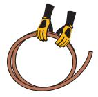
Never pull the cable over the reel flange or the side of a coil. This can produce undesirable kinks and twists in the cable.
