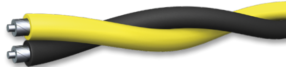
Underground/Secondary Distribution Cable (URD) - 600V Duplex, Triplex, and Quadruplex constructions available in 1350 Alloy and 8000 Series; Aluminum only
