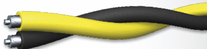
Underground/Secondary Distribution Cable (URD) - 600V Duplex, Triplex, and Quadruplex constructions available in 1350 Alloy and 8000 Series; aluminum only
