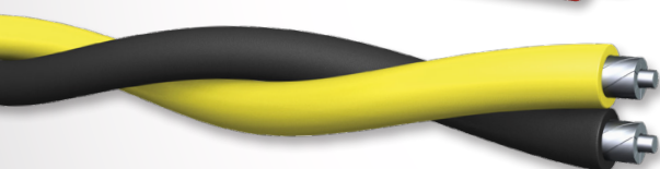
Underground/Secondary Distribution Cable (URD) - 600V Duplex, Triplex, and Quadruplex constructions available in 1350 Alloy and 8000 Series; Aluminum only
