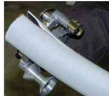
Teeth Gripping and Pulling Off Laminate Layer.
