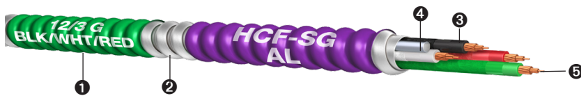
Type MC HCF-SG (SmartGround) - Copper Conductor - Aluminum Armor - THHN/THWN-2 Innere
