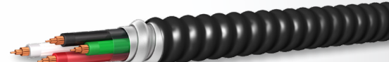
MC - PVC Jacket THWN-2/XHHW-2 Inners Available in 14 AWG-2 conductor through 750 KCMIL-4 conductor with or without a PVC jacket
