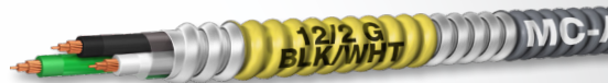
MC - THWN-2 Inners Available in 14 AWG-2 conductor through 750 KCMIL-4 conductor with or without a PVC jacket
