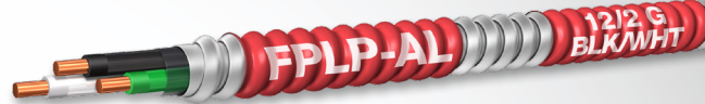
MC Fire Alarm Cable - THWN-2 Inners Available in 18 AWG-2 conductor through 12 AWG-8 conductor shielded & non-shielded; Copper only
