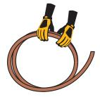
Never pull the cable over the reel flange or the side of a coil. This can produce undesirable kinks and twists in the cable.
